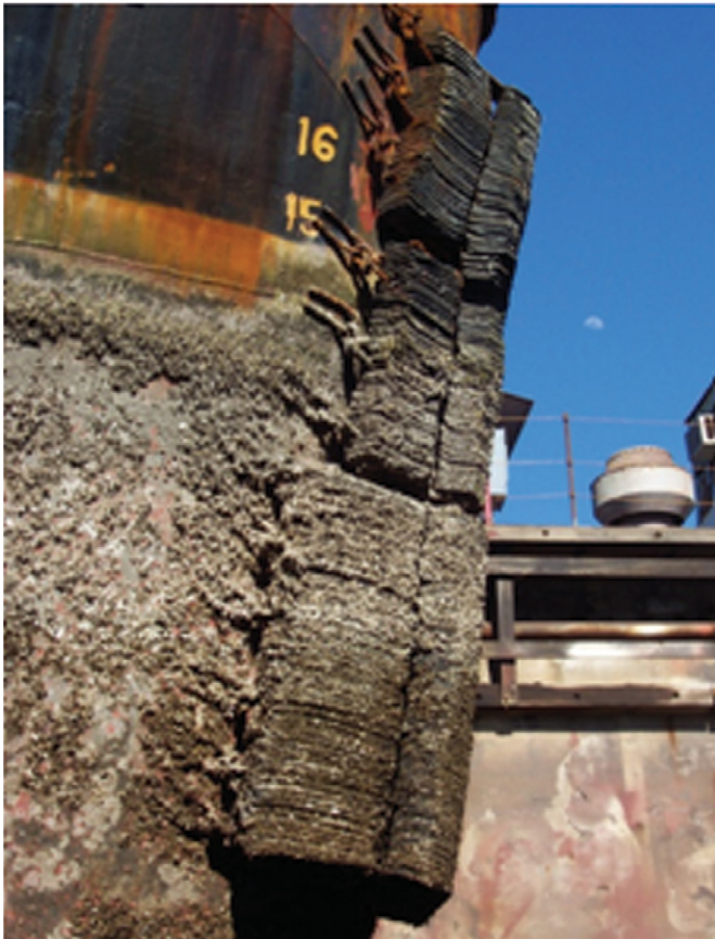
Fig. 1 Macrofouling on the hull of a ship increases drag and fuel consumption. Image courtesy of North Florida Shipyards, Jacksonville, FL.
